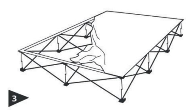
Working in a continuous direction around the frame, attach the rest of the graphic.
